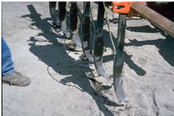
Figure 4-1-B. Shanks for injecting fumigants into the soil.
