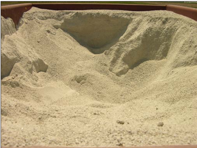
Figure 1. Photograph of typical aglime.
