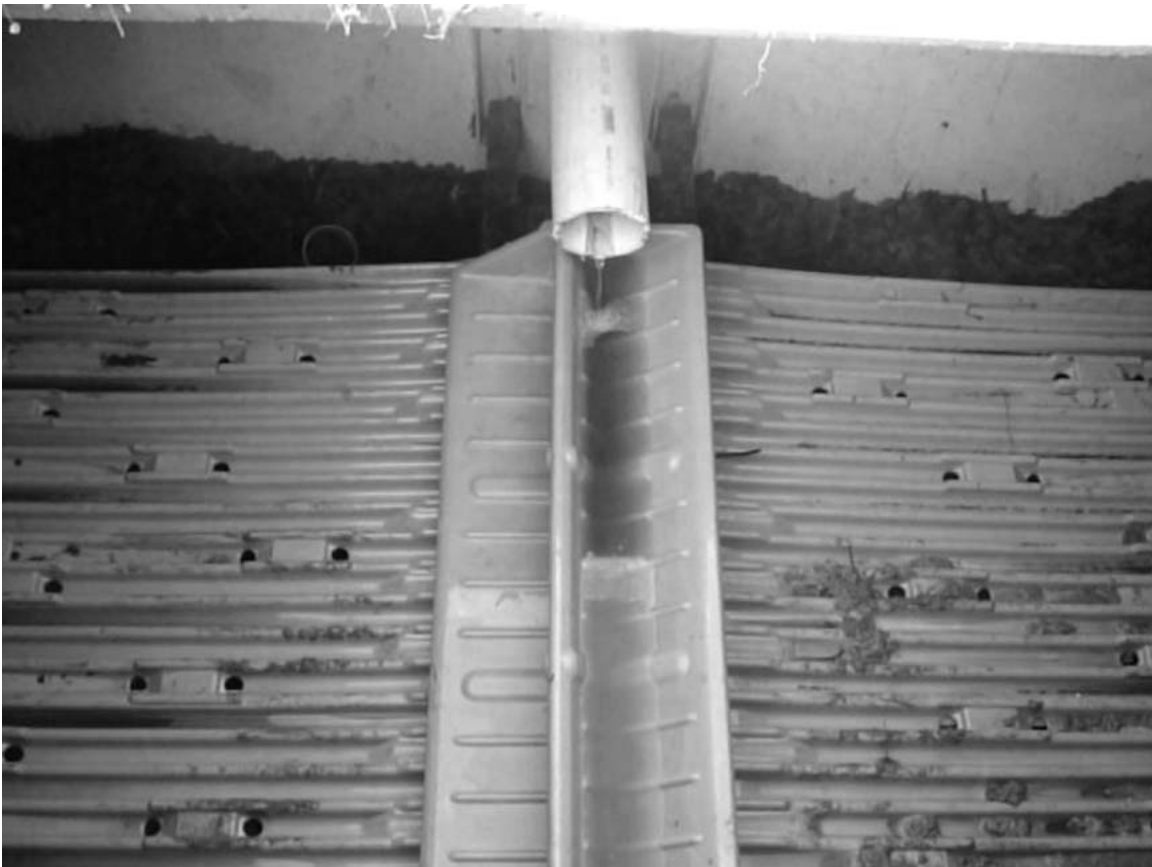
Figure 4. A tipping pan can be used for dosing wastewater onto bioreactor surfaces.
