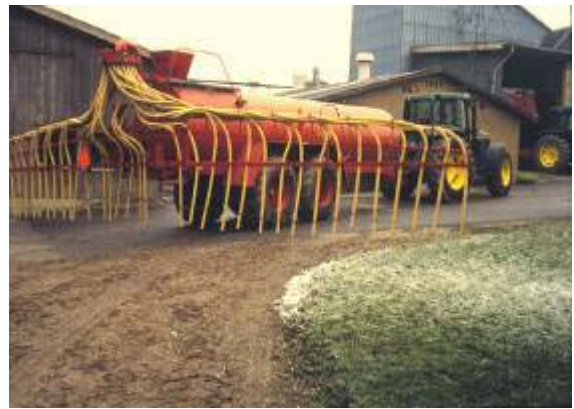
Figure 6. A European drop hoses manure applicator. (Photo © MWPS (Midwest Plan Service), Iowa State University, Ames, Iowa, www.mwps.org . Used with permission: LPES Curriculum, Lesson 44.)
